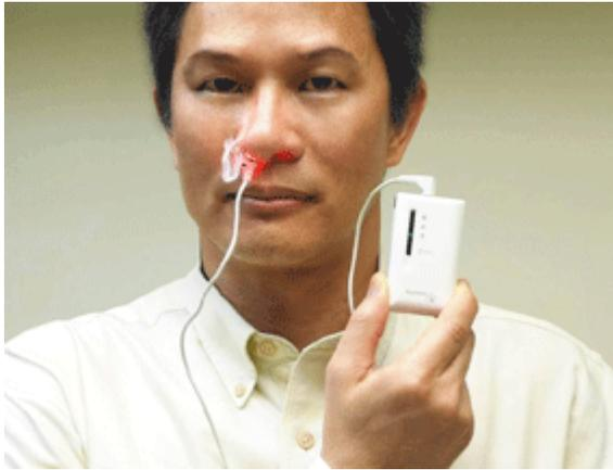
Figure 2: Intranasal light therapy device in use
